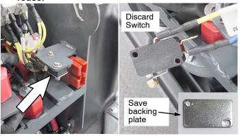
Remove the existing charger connector wire assembly from machine and discard.
