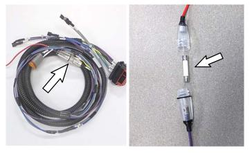
10. Install the new telemetry harness. Follow the same routing path as old harness. Connect the new telemetry harness to the following components. Secure harness with cable-ties.
