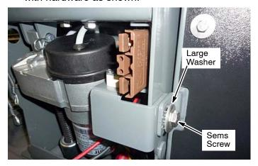
7. Route the black and red cables from the new brown charger connector up through grommet as shown.
