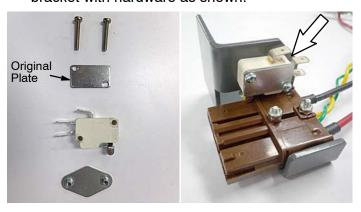
3. Plug the charger into the connector and adjust the charger interlock switch to ensure proper operation.
