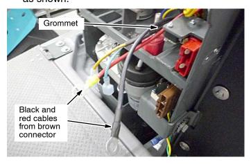
8. Connect the red cable to the (+) terminal on main contactor and the black cable to the negative stand-off.
