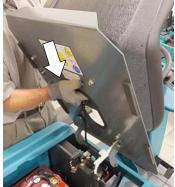
13. Reinstall fuse into telemetry harness.
